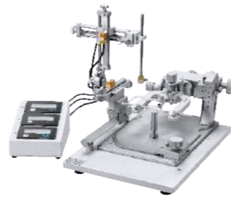
Rotational Digital Stereotaxic Instrument Easy to adjust the skull level.
