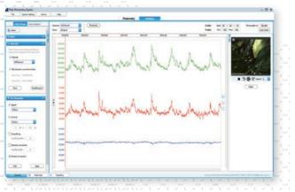
• Professional acquisition and analysis software enable stable data acquisition and easy processing. Data analysis includes data clipping, bleaching correction, smoothing, movement correction, event heat map, peak statistics, area under curve and heat map of behavior trajectory.
