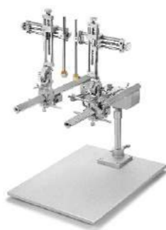
Large Animal Stereotaxic Instrument Used to stereotaxic experiments of cats, dogs, monkeys and other large animals.
