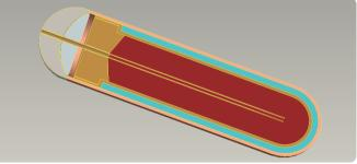
The RWD Osmotic Pumps consist of three concentric layers: the inner drug reservoir the osmotic layer, and the outer. When the pump is implanted water is absorbed through the outer membrane. The water entering the pump expands the osmotic layer, which compresses the flexible, impermeable reservoir.
