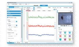
Professional acquisition and analysis software enable stable data acquisition and easy processing. Data analysis includes data clip, smoothing, baseline correction, motion correction, event heat map, peak statistics, area under curve, behavior trajectory heat map and fluorescence-place heat map.
